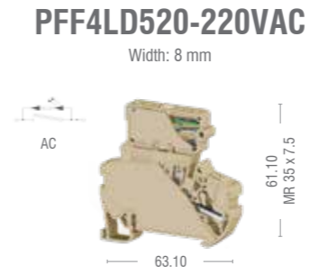
PFF4LD520-220VAC Width: 8 mm 4 mm² Fuse Modular PushFit Feed Through Terminal Block 5x20 Fuse, 220 VAC with LED For 35 mm DIN Rail
