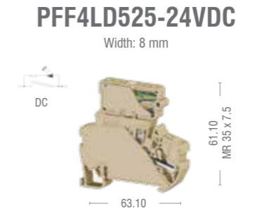
PFF4LD525-24VDC Width: 8 mm 4 mm² Fuse Modular PushFit Feed Through Terminal Block 5x25 Fuse, 24 VDC with LED For 35 mm DIN Rail
