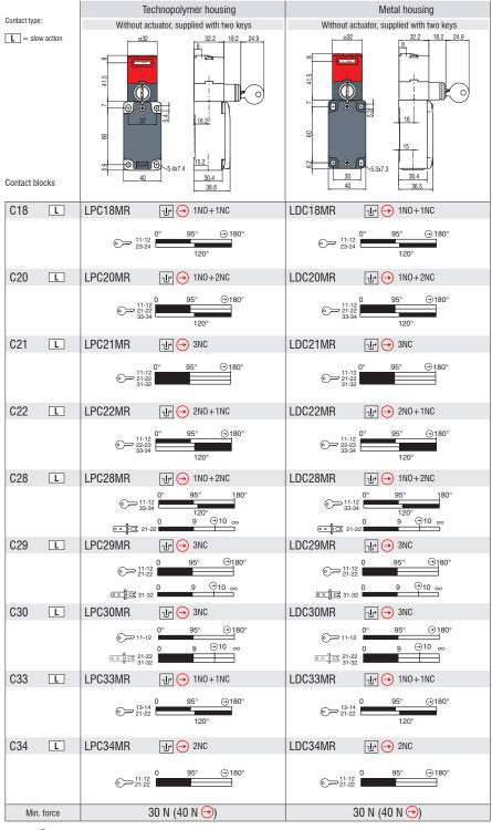
Legend: With positive opening according to EN 60947-5-1, 1 interlock with lock monitoring in accordance with EN ISO 14119
