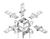
The head can be quickly turned to each of the four sides of the switch by unfastening the two fixing screws.
