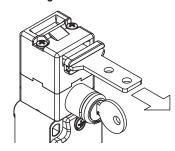
The inside of each switch features a device which holds the actuator in its closed position. Ideal for all those applications where several doors are unlocked simultaneously, but only one is actually opened. The device keeps all the unlocked doors in their position with a retaining force of 30 N~, stopping any vibrations or gusts of wind from opening
