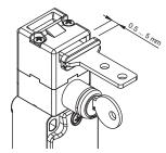
The head of this switch has been designed to have a certain amount of movement tolerance for oscillation along the direction of insertion without causing unwanted machine shutdown caused by switch activation. This feature is available with all interlock actuators, in order to ensure maximum device reliability.
